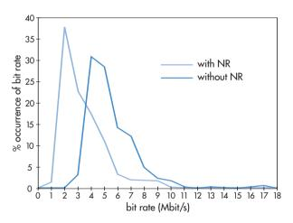
have on the efficiency of an MPEG coder. Two encoders are working with fixed coding quality and variable bit-rate on a typically noisy source. A histogram of the occurrence of different bit rates is shown for each encoder. Encoder 2 has no pre-processor while encoder 1 has pre-processing. This simple example shows that preprocessing can easily be worth 2 Mbit/s per channel on fairly typical material.
