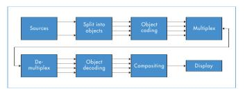
Video information is coded separately as synthetic or natural objects, and the resulting bitstreams are multiplexed together. The decoder contains a *compositor* which puts the decoded objects back together, under the control of instructions which are either decoded from the bitstream or over-ridden by input from the user, providing a measure of interactivity.
